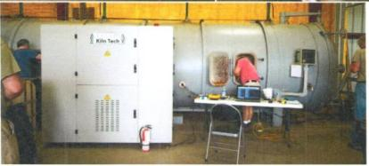
and could potentially run up to 10 cycles or 5,900 GMA pallets per day. An automated tram system for the RF chamber facilitates faster loading and unloading that appears to be less than typical dry kiln loading/unloading times of 1 to 1.5 hours.
